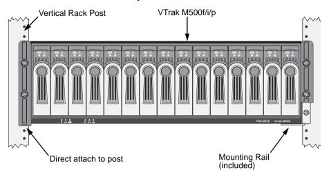
Figure 1. Rackmounted VTrak M500f/i/p
